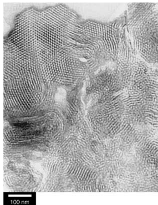
Figure 2. TEM image of ZSM-5-coated MesoAS.
